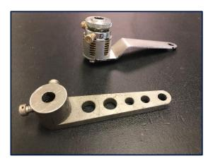
Install the replacement arm by sliding the clutch mechanism over the servo motor shaft with the arm in the same position. Make sure the arm is closest to the servo motor.
