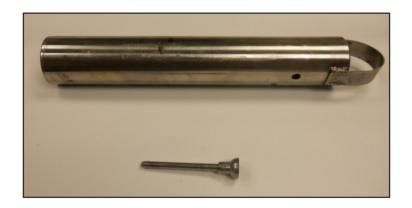
It is critical that the ballast be positively secured when placed in the carrier in the tail boom. The current Safari Kit supplies a Quick Lock Pin which is adequate to secure the ballast if it and the carrier are in good working order.
